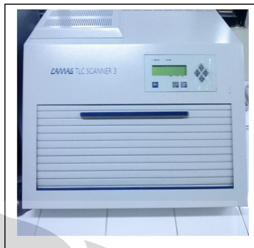
Gambar 3.2 TLC Scanner III (Camag)
