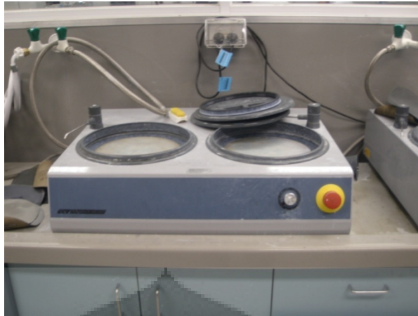
Figure 3.10: Grinding apparatus with two rotating disk and rotation speed control.
