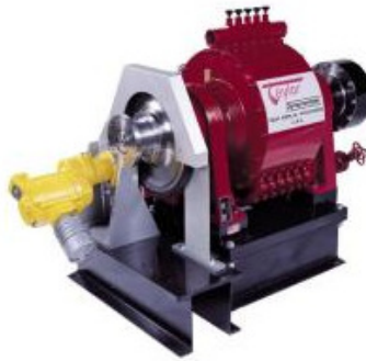
Gambar 2.7 Dynamometer Water Brake
