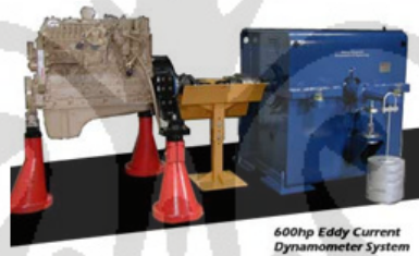
Gambar 2.8 Dynamometer Eddy Current
