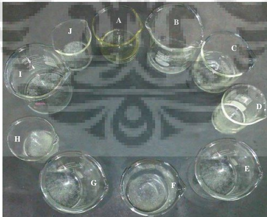
Gambar 4.5. Kelarutan kitosan asal pada larutan pH : 1,2 (A); 3,0 (B); 5,0 (C); 6,0 (D); 7,4 (E); 8,0 (F); 9,0 (G); 10,0 (H); 12,0 (I) dan 14,0 (J).
