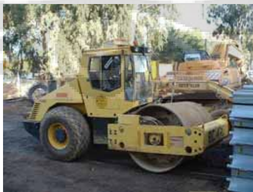
Gambar 2.3. 4 Vibrator roller (road roller)
