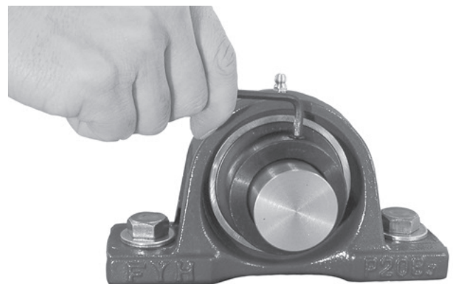
Fig. 14.10 Installing eccentric locking collar
