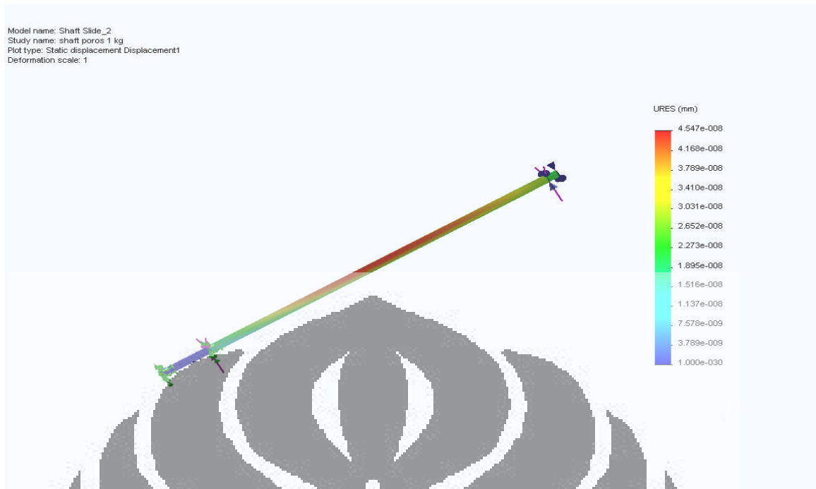
Gambar 3.35. Hasil analisis diplacement poros vertikal
