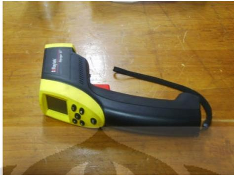
**Gambar 3.3** Termometer *infra-red*
