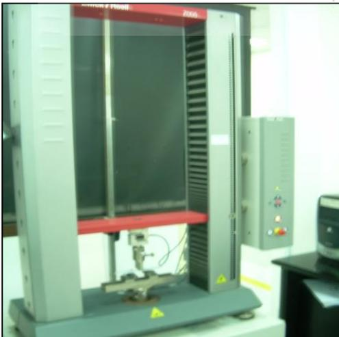
**Zwick/Roell Multi-Testing Machine** with Compression Load Cell & Support Span Computerized (O.S.: Windows XP)
