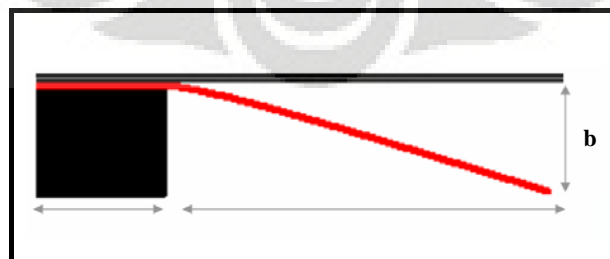
Figure III.3 : Schematic diagram of deflection test
