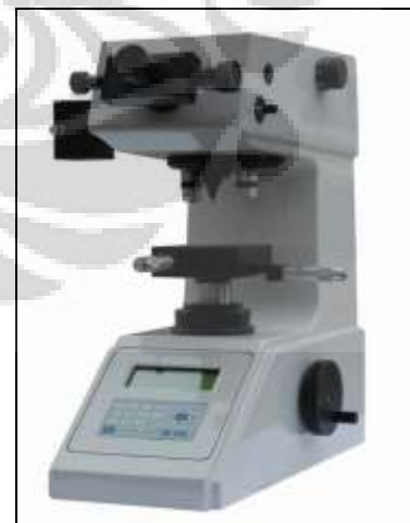
Gambar 3.10.b Micro Hardness Testing
