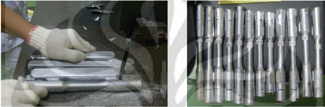
Gambar 3.5 a) proses cutting sampel uji tarik; b) hasil sampel uji tarik
