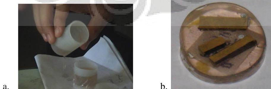
**Gambar 3.8** a. Contoh cetakan mounting, b. Hasil mounting.
