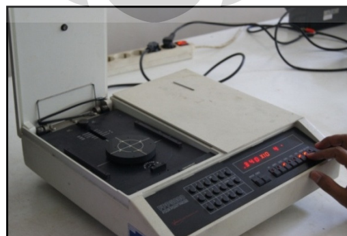
Gambar 3.7 Mesin Veeco FPP 5000 - Four Point Probe Test
