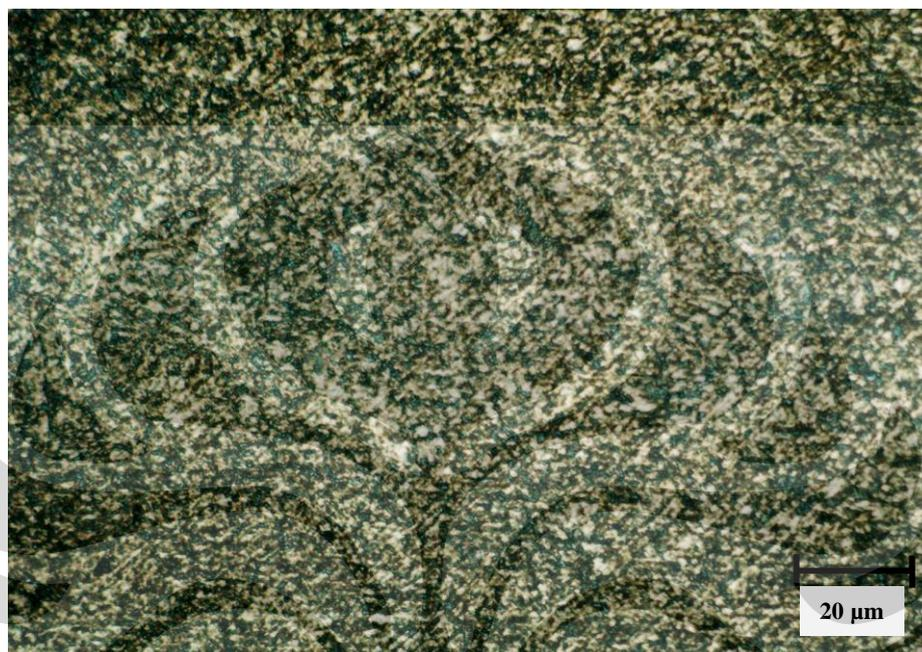
**Gambar 4.6** Struktur mikro sampel *austemper* 10 menit. Nital 2-3%. 500x
