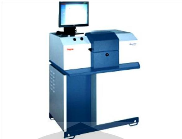
**Gambar 3.5** *Optical emission spectrometer (OES)*
