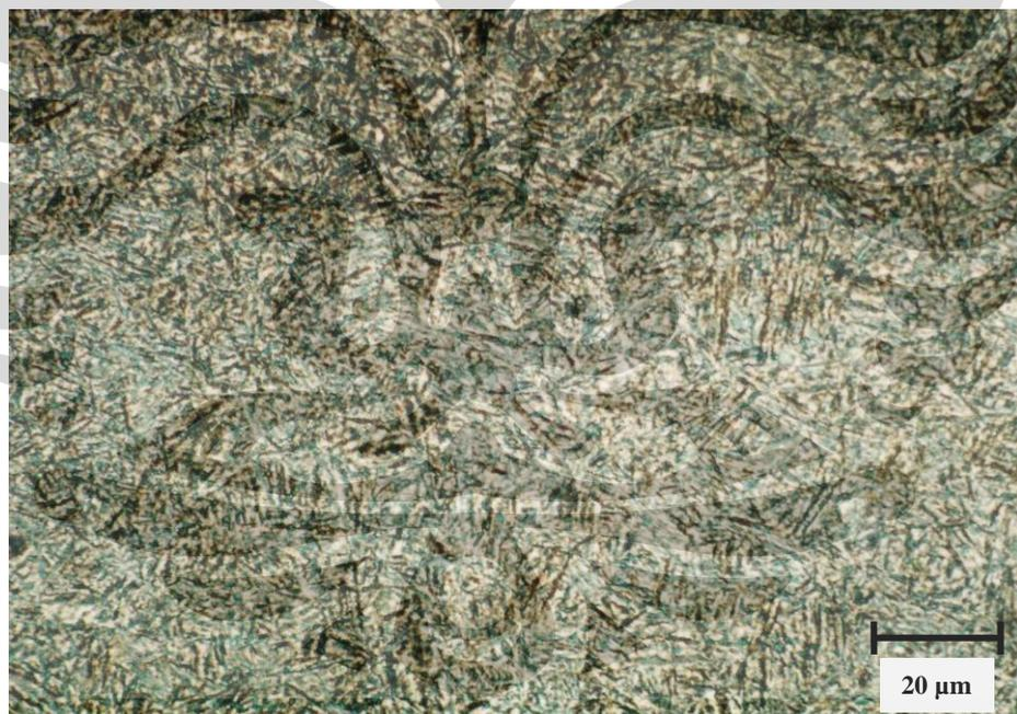
**Gambar 4.10** Struktur mikro sampel *austemper* 20 menit. Picral 15%. 500x
