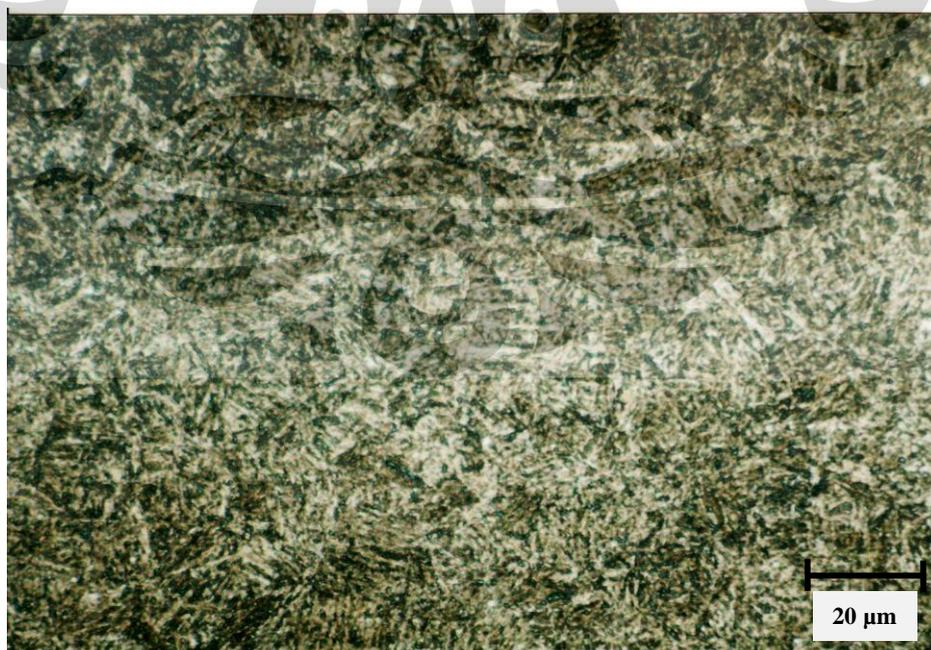
**Gambar 4.7** Struktur mikro sampel *austemper* 20 menit. Nital 2-3%. 500x
