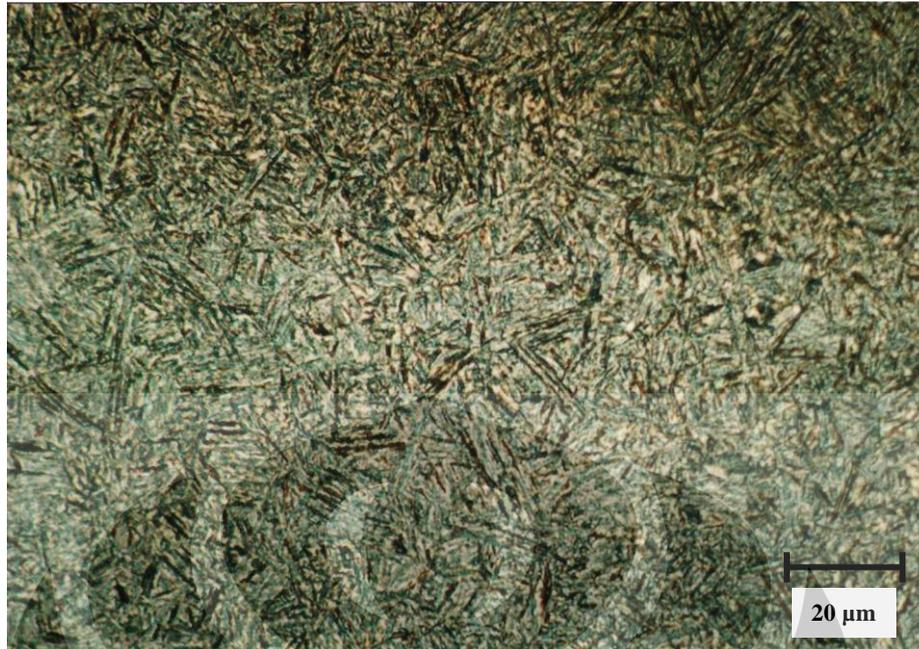
**Gambar 4.11** Struktur mikro sampel *austemper* 30 menit. Picral 15%. 500x
