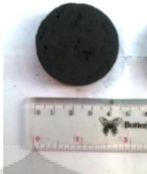
**Gambar 4.2** Material komposit grafit-coal tar pitch hasil sinter
