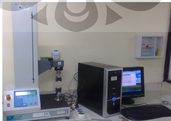
Gambar 3.22. Alat uji tarik plastik LF Plus Series Digital.
