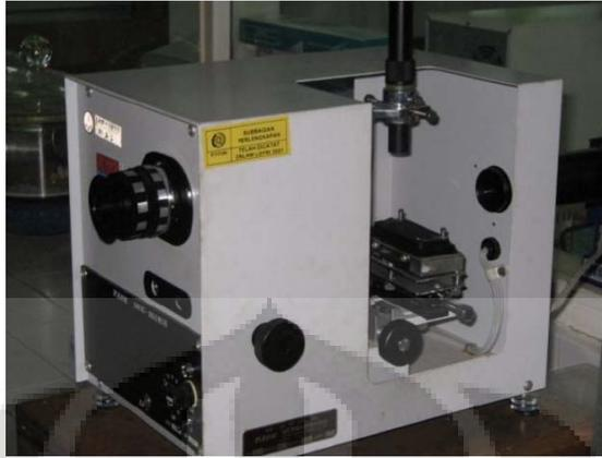
Gambar 3. 4 Alat Contact Angle Meter
