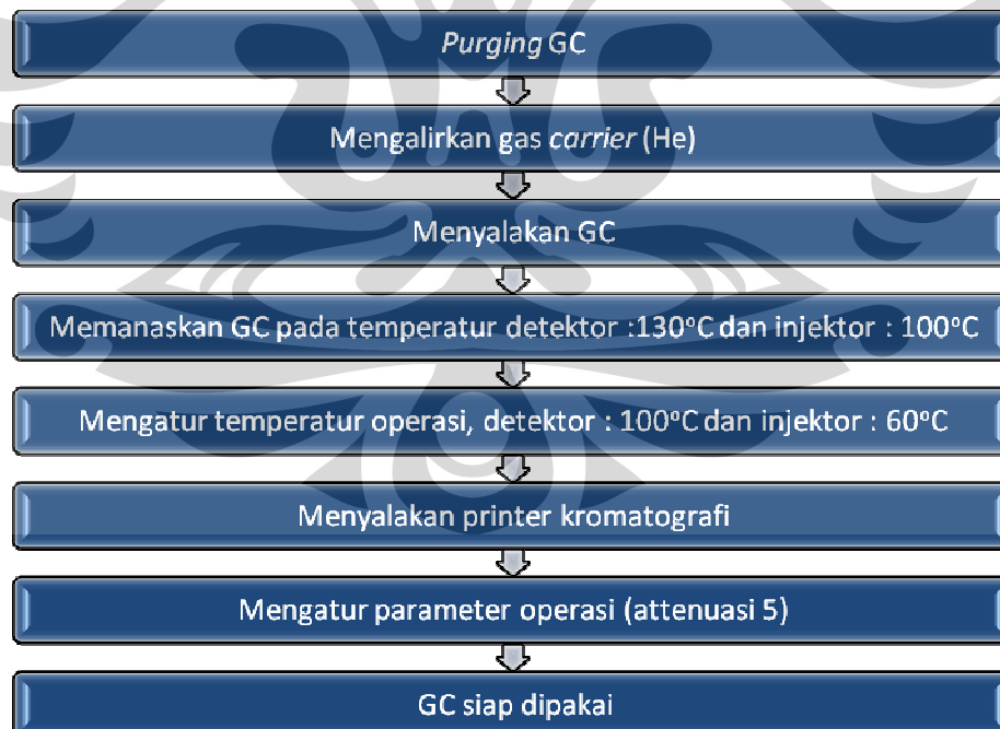
Gambar 3.9 Diagram alir prosedur pengoperasian GC
