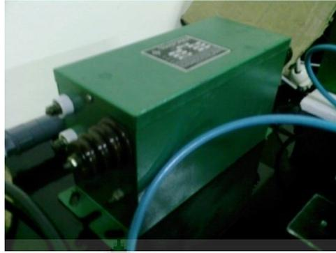
**Gambar 3.11** Neon Sign Transformer
