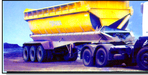
Gambar 3.3 Side Dump Tipper Semi Trailer
