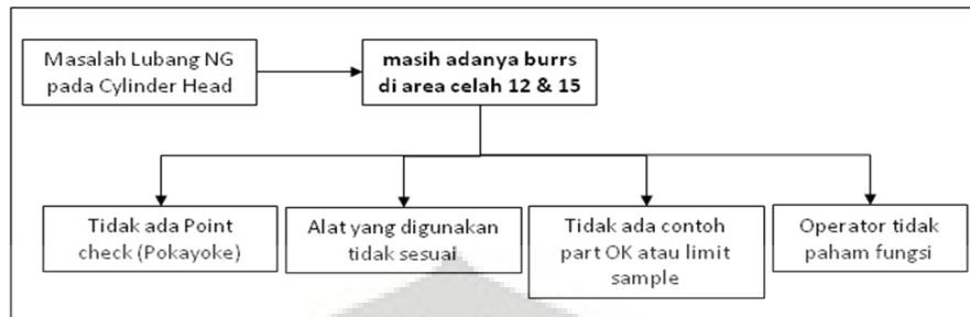
Gambar 4.7 Failure Tree Analysis Proses Trimming
