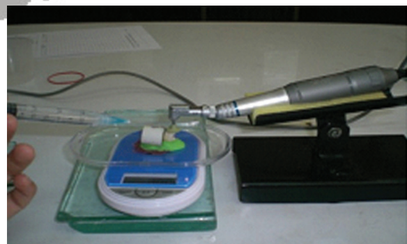
Figure 1. Polishing procedure using either one-step polishing system (OpraPol) or multi-step polishing system (Astropol)
