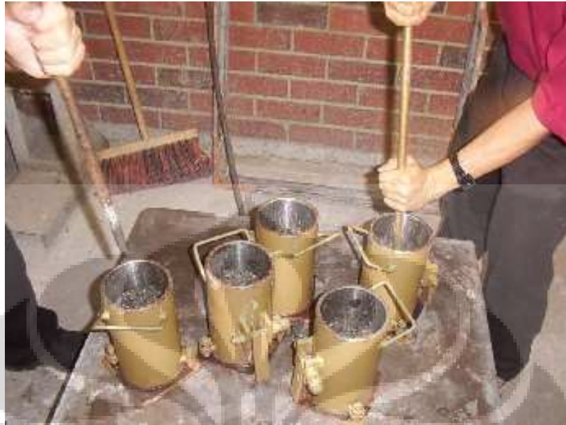
Figure 3.12: Compaction into Moulds
