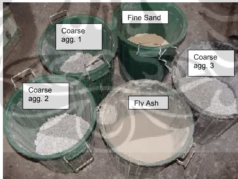
Figure 3.8: Dry Materials for Making Geopolymer Concrete
