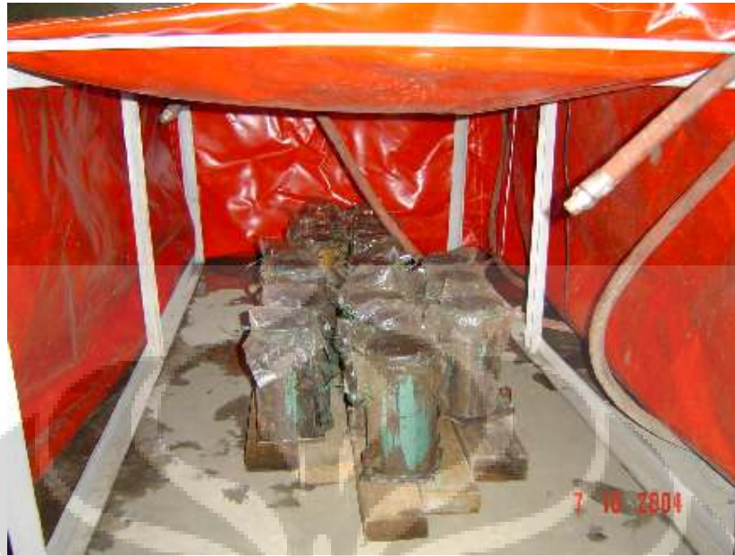
Figure 3.14: Specimens in Steam Curing Chamber
