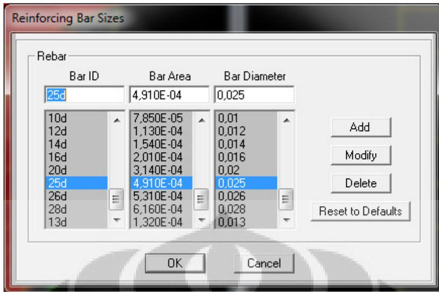
Gambar A4. Reinforcing Bar Sizes
