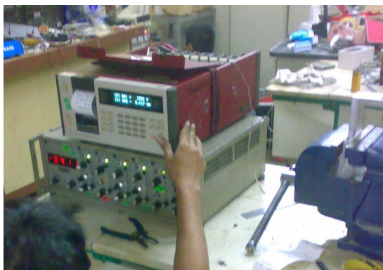
Gambar 4.2 Instalasi Data Logger
