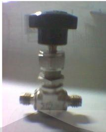
Gambar 3.9 *Needle valve* SS-ORS2
