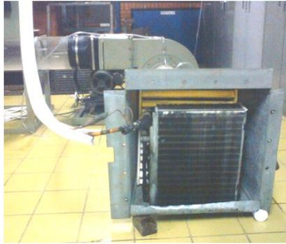
Gambar 3.4 evaporator dan drift eliminator
