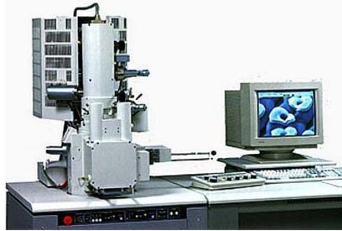
**Gambar 2.23 Scanning Electron Microscope (SEM) [27].**
