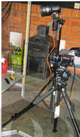
**Gambar 4.7** *High Speed Video Camera*
