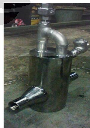
Gambar 3.3 Proses manufaktur *evaporator*
