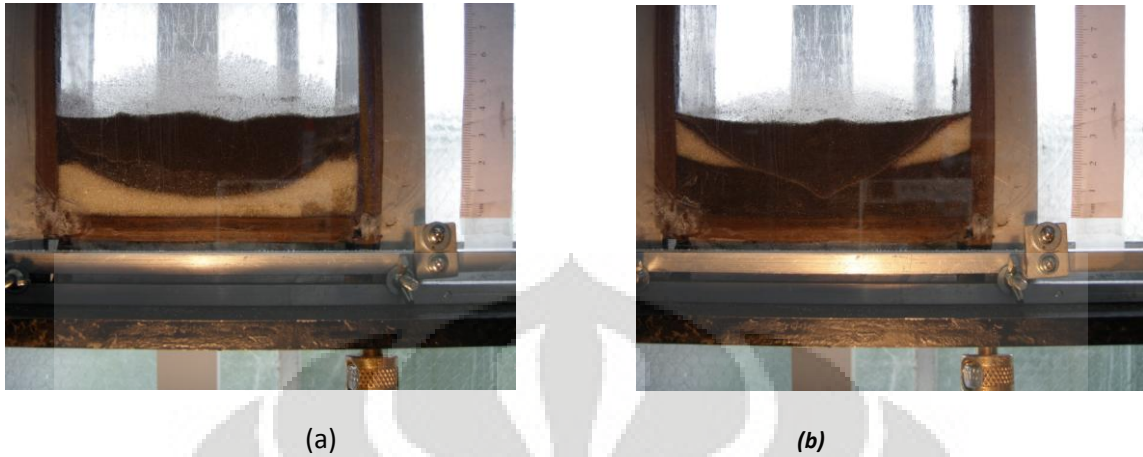
Figure 4.2. The comparison of particle arrangement between straight wall fluidized bed at 4 cm with binary particles of 106 – 212 microns and 355-425 microns at bubbling flow rate (a: coarse particle placed on the bottom, b: coarse particle placed on the top)
