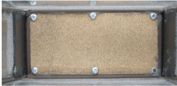
Figure 4.11. Top view of inside the fluidized bed with empty bed
