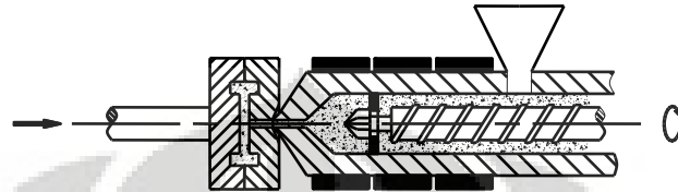
Gambar 2.8 Langkah Kerja Mesin Injeksi 3 (Sumber : Menges Mohern, How to Make Injection Mold , Hansen Pablisher, 1986)
