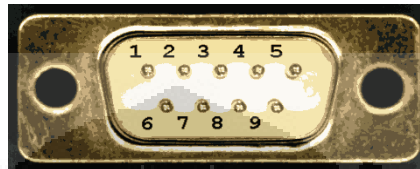
Gambar 2.9. Urutan Letak Pin Female RS232 DB-9
