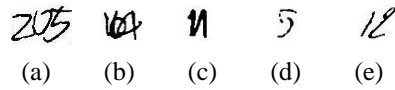
Fig. 2. Different problem types for digit segmentation: (a) touching, (b) overlapping, (c) surplus stroke connection, (d) broken, and (e) slanted digits.
