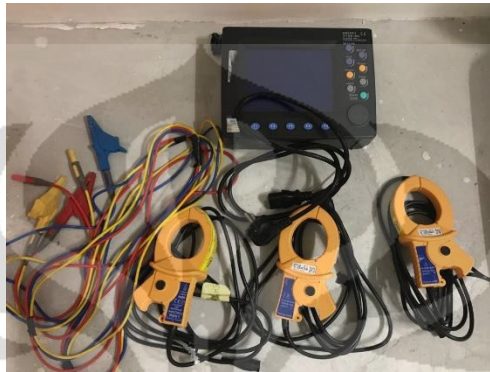
Gambar 3.10 alat Power Quality Analyzer
