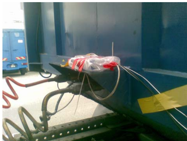
Figure 7 Dewe-soft device installation on the truck chassis
