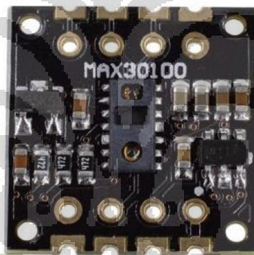
Gambar 2. 3 Modul sensor Max 30100
