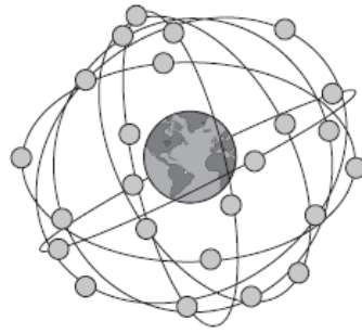
Gambar 2.10 GPS Satellite Constellation
