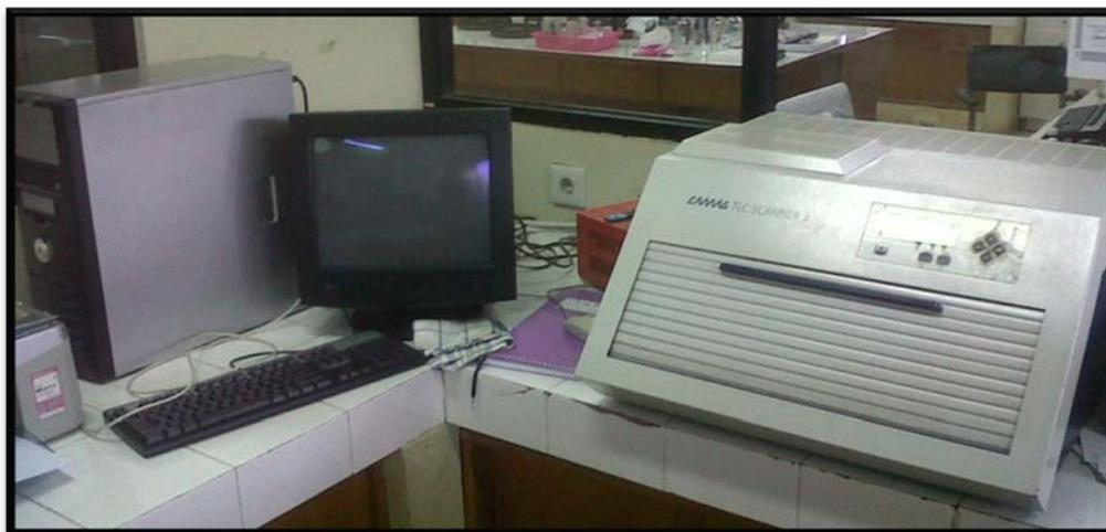
**Gambar 4.20.** Alat KLT Densitometri (*TLC Scanner Camag*)
