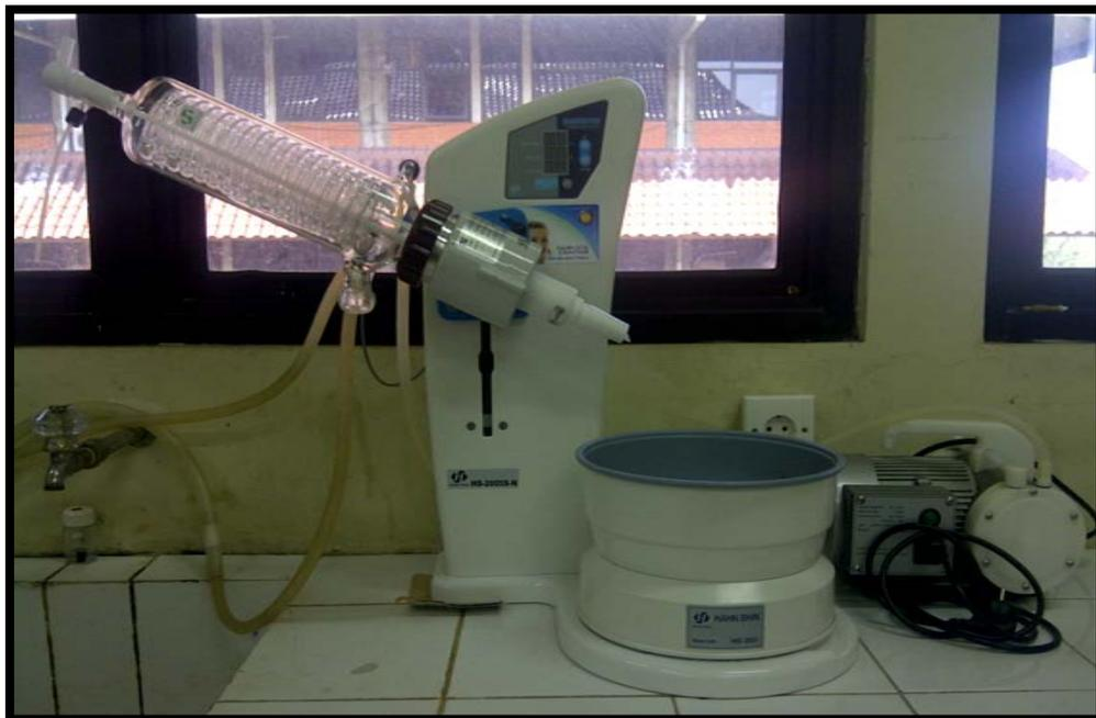
**Gambar 4.18.** Alat *Rotary Evaporator Vacuum* Hahn Shin
