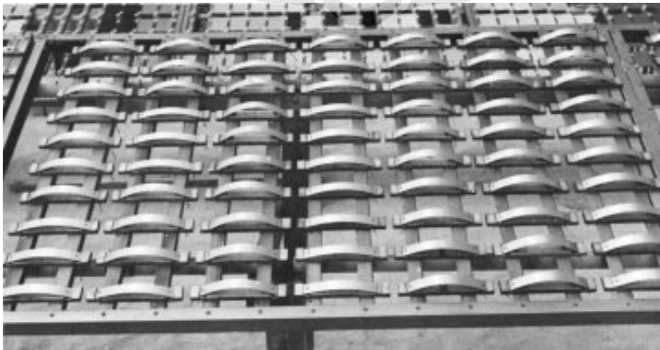
FIG. 4 Bent-Beam Specimens on Atmospheric Exposure Rack
