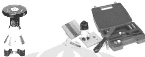
**Gambar 3.8.** Peralatan *Elcometer Model 106 Adhesion Tester*
