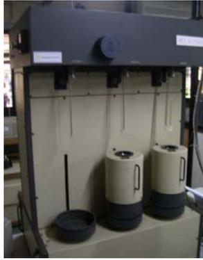
**Gambar 2.13.** Mesin BET surface area
