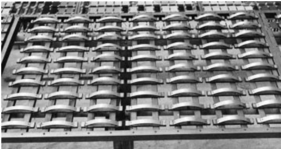
FIG. 4 Bent-Beam Specimens on Atmospheric Exposure Rack
