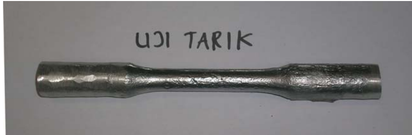
Gambar 3.12 (a) Standar sampel tarik ASTM E-8 [25] (b) Sampel Uji Tarik
