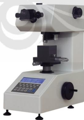
**Gambar 3.7** Vickers microhardness tester
