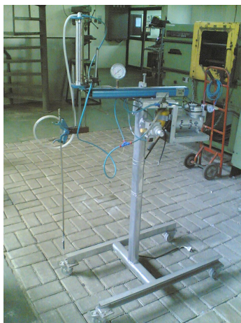
Gambar 3.4 Peralatan uji fluiditas metode vacuum suction test
