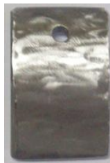
Gambar 3.1 Kupon Baja ASTM A53
