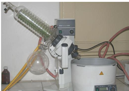
**Gambar 6.** Rotavapor-vacuum pump-waterbath Büchi
