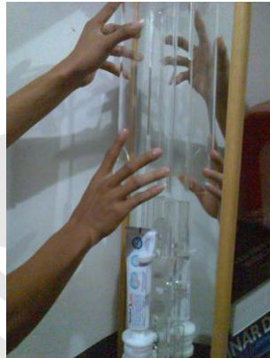
Gambar III.25 :Melepas casing Pump Toothpaste Dispenser
