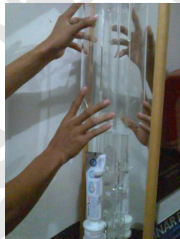
Gambar III.21 : Cara menutup casing Pump Toothpaste Dispenser
